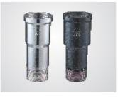
**Bottom adaptor:** This is a metal accessory, that is used to connect the first piece of uPVC column pipe to the submersible pump. As explained, to enable higher load bearing capacity, C.R.I. column pipes are equipped with square threads. Whereas, the submersible pumps are generally with V threads. Since, the joint cannot be made due to various threads and pitches, an adaptor is used.
