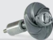
**Cutting Device:** cutting device suitable to reduce into little pieces solids contained into liquids. This device permit the use of small pipes without risk of clogging. Either the fixed part and the movable are built in a special stainless steel.
