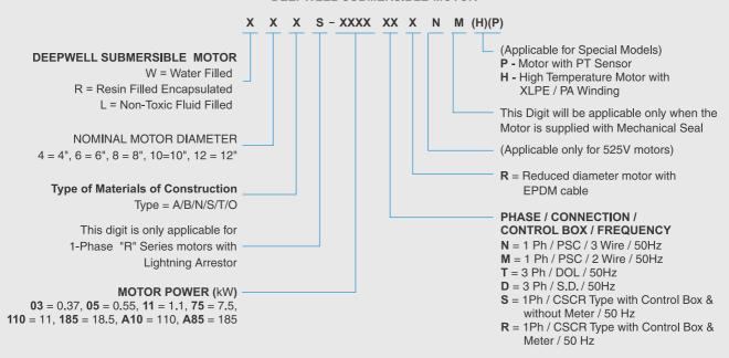
DEEPWELL SUBMERSIBLE PUMP SET (Pump + Motor) PUMP MODEL + MOTOR MODEL S X X - XXX / XX + X X X - XXX X DEEPWELL SUBMERSIBLE PUMP SET (Pump + Motor) **PUMP MODEL** + MOTOR MODEL S6S - 18 / 03 W6A - 22 T
