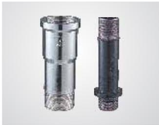
**Top adaptor:** This is a metal accessory, that is used to connect the last piece of uPVC column pipe to the outlet / discharge bend. As explained, to enable higher load bearing capacity, C.R.I. column pipes are equipped with square threads. Generally, the outlet / discharge bend, are with V threads. Since, the joint cannot be made due to various threads and pitches, an adaptor is used.
