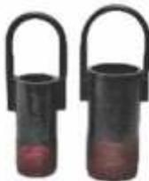
**Lowering Jig:** It is an accessory which is used to lower the pipe in the borewell. The male end of the Lowering Jig is with square threads to fit into the pipe and the other end is provided with a hook, which can be tied up to the chain of the tripod stand, enabling easier lowering of the pipes.
