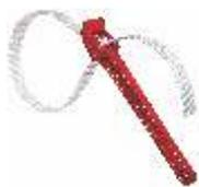
**Belt Wrench:** It is a type of wrench used to tighten the uPVC column pipes. Since chain wrenches cannot be used on the uPVC column pipes, belt wrenches are recommended.
