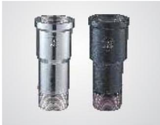
**Bottom adaptor:** This is a metal accessory, that is used to connect the first piece of uPVC column pipe to the submersible pump. As explained, to enable higher load bearing capacity, C.R.I. column pipes are equipped with square threads. Whereas, the submersible pumps are generally with V threads. Since, the joint cannot be made due to various threads and pitches, an adaptor is used.
